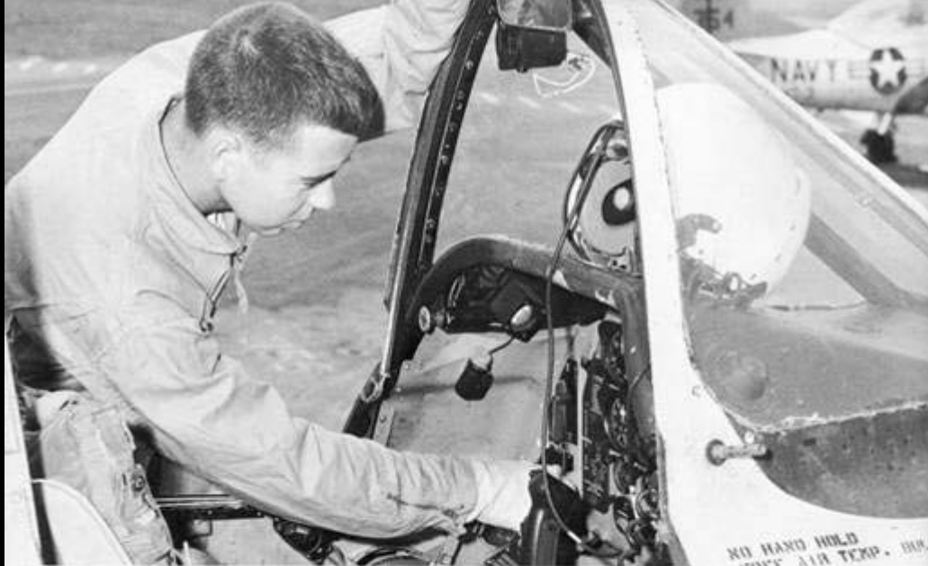
Landing gear handle is checked for correct position by VT-3 student.
