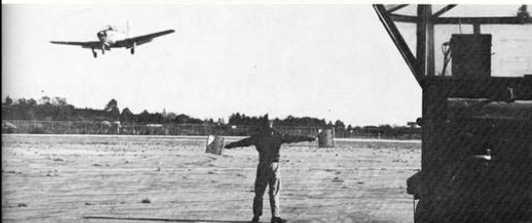
A training Squadron One student returns from a solo flight and is guided to a landing by the Landing Signal Officer, who has two means of communicating to the pilot: (1) Brightly colored flags indicates his gear is down and locked, and (2) Radio transmitters and receivers (in the truck) to talk to the student.
