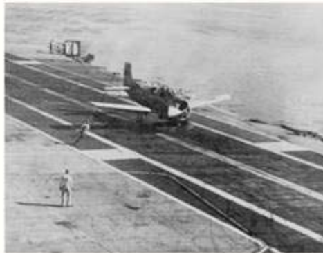
Student catching a wire on an arrested landing of the carrier.
