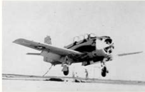
Student catching a wire on an arrested landing of the carrier.
