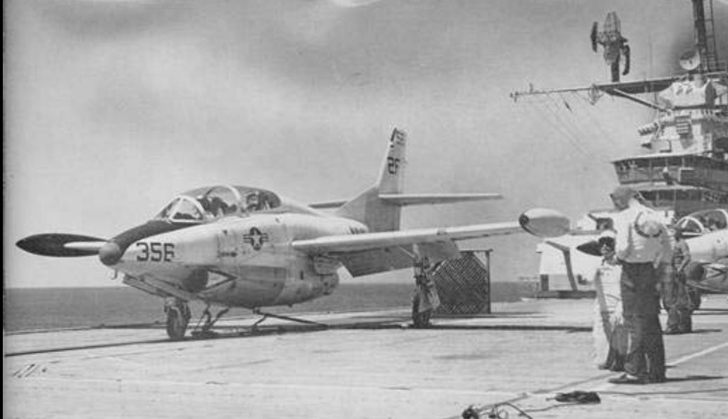
A T2J jet trainer ready to be catapulted from the starboard catapult.
