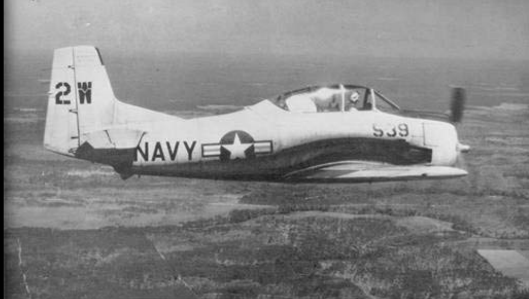
During an instrument flight from Whiting, a student flies this T-28 while under the hood in the rear cockpit. The hood is used to prevent the student's reference to the ground.
