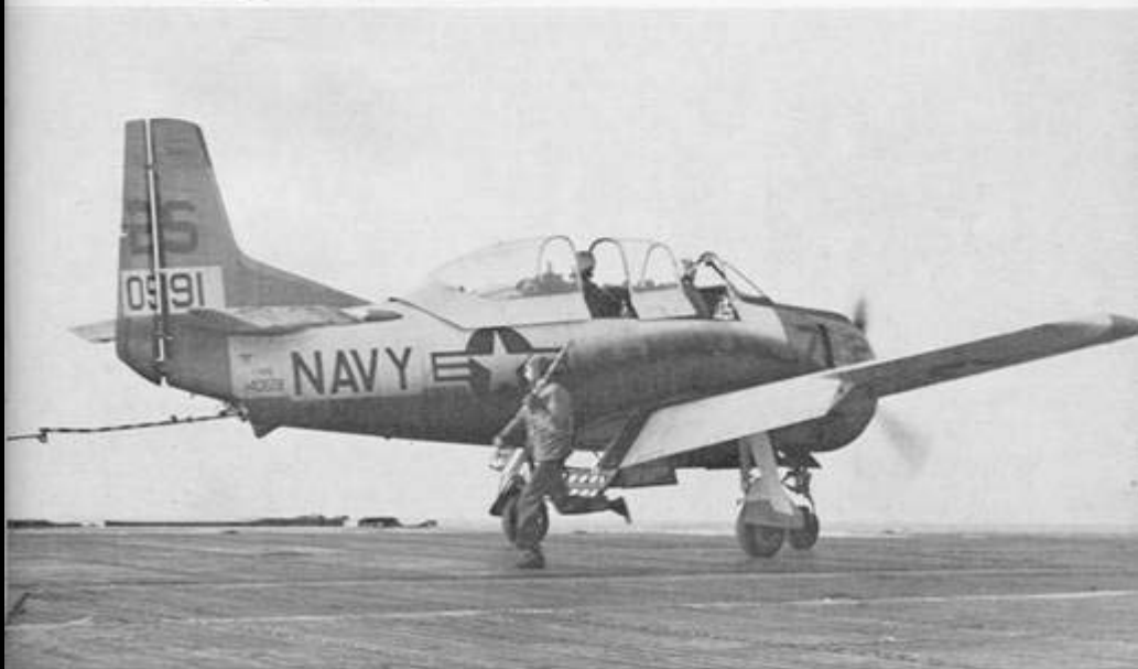
A T-28C comes to a complete stop after being arrested by one of the six arresting cables. The hookrunner disengages the cable from the hook.
