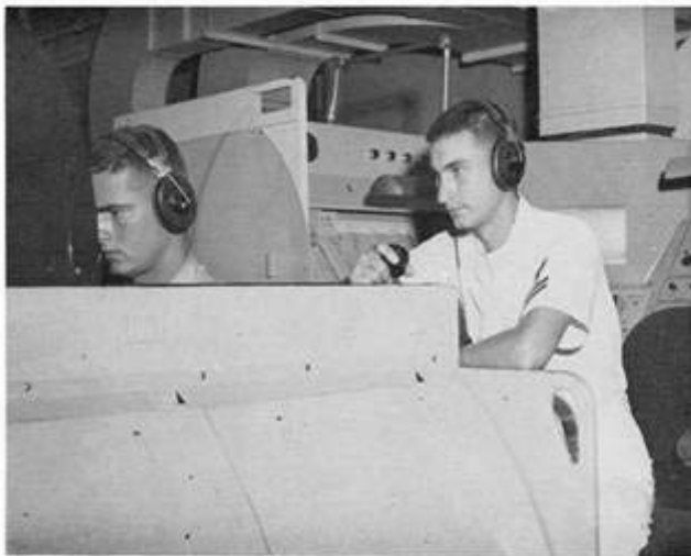
The link trainer is a duplicate of the T2V Sea Star's cockpit. All students fly the links on instruments for as many hours as they fly in the air. The link trainer not only facilitates training, and simulates actual flight realistically but saves the Navy countless dollars in the overall cost of training students.
