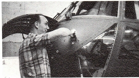
One modification was SAS drain covers
